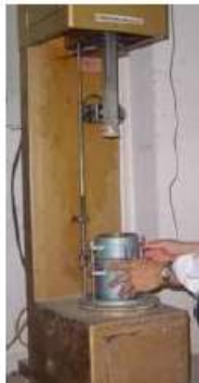
In the lab increasing compaction energy = increasing number of blows
