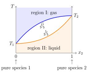
Figure 8.1: An isobar phase diagram of a typical binary solution. For the pressure considered,  $T_1$  is the liquid/gas coexistence temperature of species 1 alone and  $T_2$  is the liquid/gas coexistence temperature of species 2 alone.
