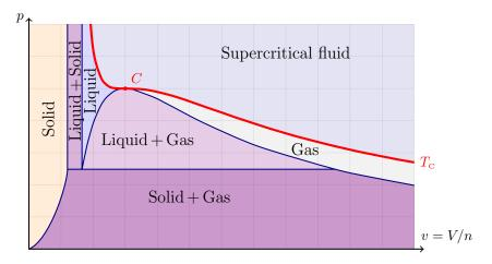
Figure 7.6: Coexistence regions of the solid, liquid and gas phases in a pressure-volume diagram.
