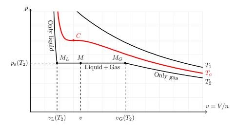
Figure 7.4: Three isotherms in a (p, v) diagram. The pressure plateau indicates the coexistence of the liquid (L) and gaseous (G) phases.
