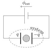
A system made of a sample placed between the armatures of a capacitor is considered. A voltage  $\phi_{\text{ext}}$  is applied to this capacitor by a generator; it is this generator (placed outside the system) that delivers the work. During a transformation that, for example, changes the capacity of the capacitor, the electric charge on its plates changes. The work received is then
