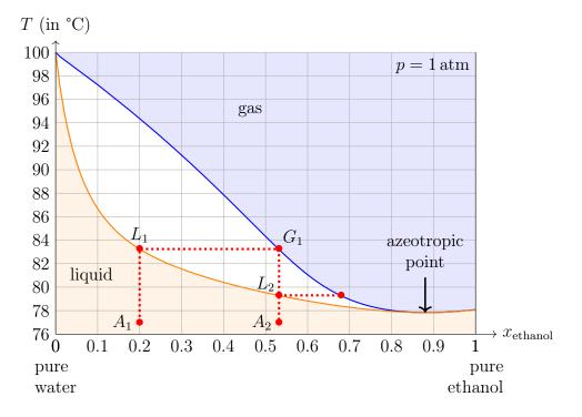
Figure 8.3: Principle of distillation.
