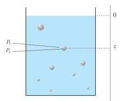
Schematic of boiling in a liquid.
