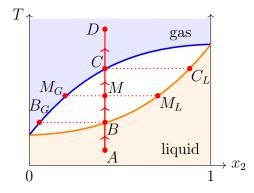
Figure 8.2: Heating a liquid binary solution.
