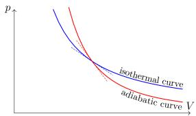
Comparison of isothermal and adiabatic curves in the Clapeyron diagram.
