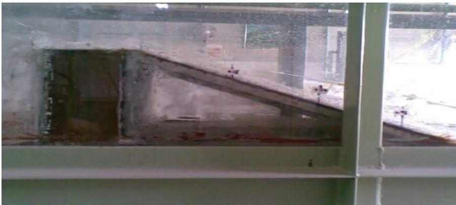
Figure 2. The Submerged dams supported by inclined plan
