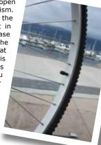
remove one side of the tire only to allow the tube to be exposed for repair.
