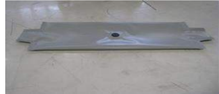
Figure 2.3: A 30 L laboratory-scale textile-based bioreactor prototype.
