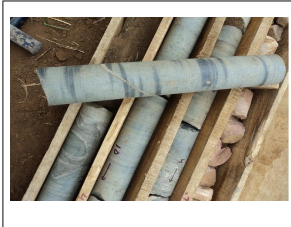
Figure 1.5: NX sized core obtained after drilling.
