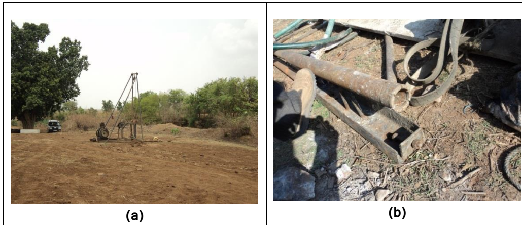
Figure 1.4: (a) Diamond core drilling setup. (b) Diamond drill core barrel for NX size cores
