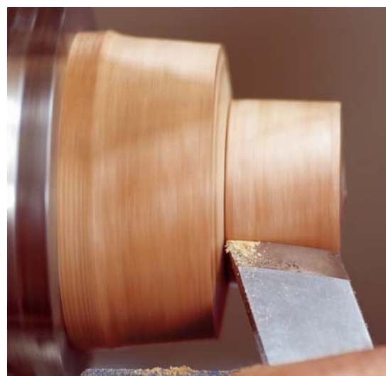
A curved edge skew is particularly useful for delicate low-peeling cuts. Here the long point reaches into the corner without touching the rest of the surface.
