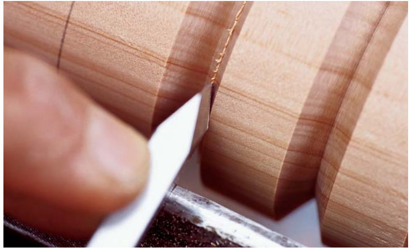
When cutting a groove, only the bevel side and the long point of the skew chisel should contact the wood.
