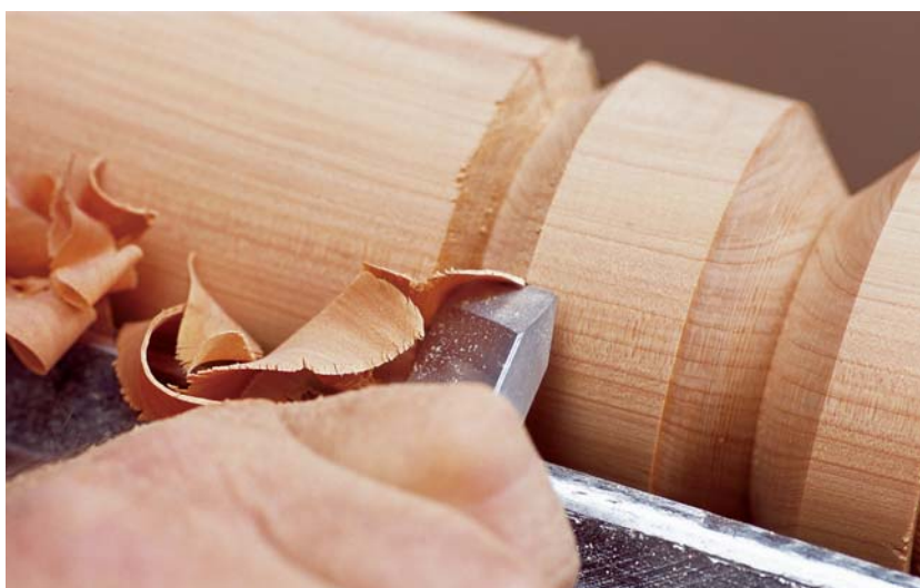
The skew chisel can be used to rotary-peel on an angle by pivoting the tool into the wood diagonally. To avoid a catch, you must be quick to rotate the edge clear at the end of the cut.
