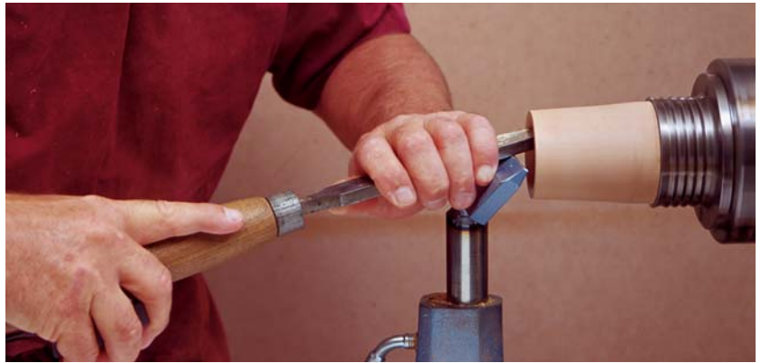
The large round-nose scraper is tilted upwards to shear-cut as I begin smoothing an internal curve.
