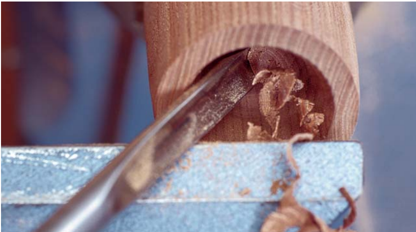
Back-hollowing cuts start at center and heads away at 1 o'clock to 3 o'clock.
