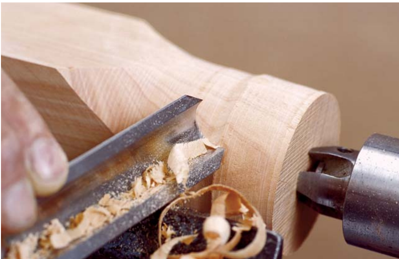
Scooping cuts using a 1-in. (25mm) deep-fluted roughing gouge reduce the square section blank to round.
