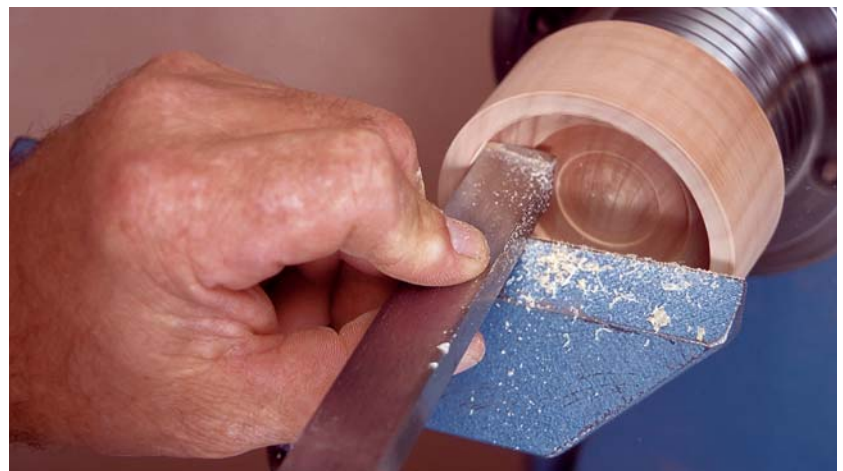
A \frac{3}{4} -in. (20mm) square-edge scraper is used to cut a cylindrical flange in a box lid.
