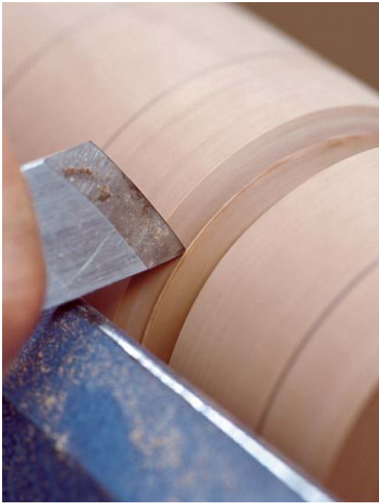
Use the skew chisel long point down when cutting grooves.
