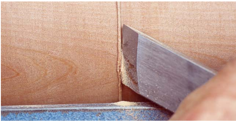
(TOP) Cutting with the long point down allows you to steer the tool in the direction you're cutting. Tool chatter is reduced because pressure against the axis is minimal, and any force in the cut is absorbed by the headstock. (BOTTOM) If the tool is pointing in the right direction but with the long point up, it won't cut because the vertical edge butts into end grain.
