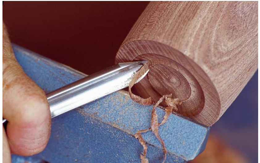
Hollowing end grain from the rim.
