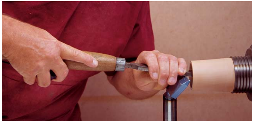
Using scrapers on end grain, raise the tool rest so that as you start a cut at center, the tool tilts down a few degrees. For a flowing internal curve, ease your elbow down on the handle and don't move the tool forward on the rest.
