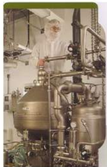
Fig. 26.2: Continuous centrifugation wherein the media and cells get in & clarified media go out
