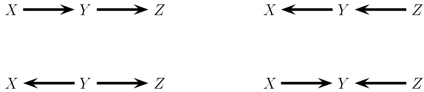
FIGURE 20.5. The first three DAG's have no colliders. The fourth DAG in the lower right corner has a collider at Y .
