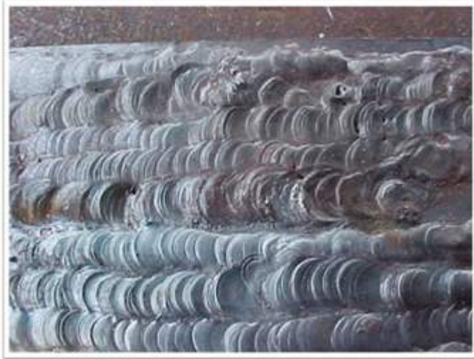
Figure 7.23 unacceptable weld profiles
