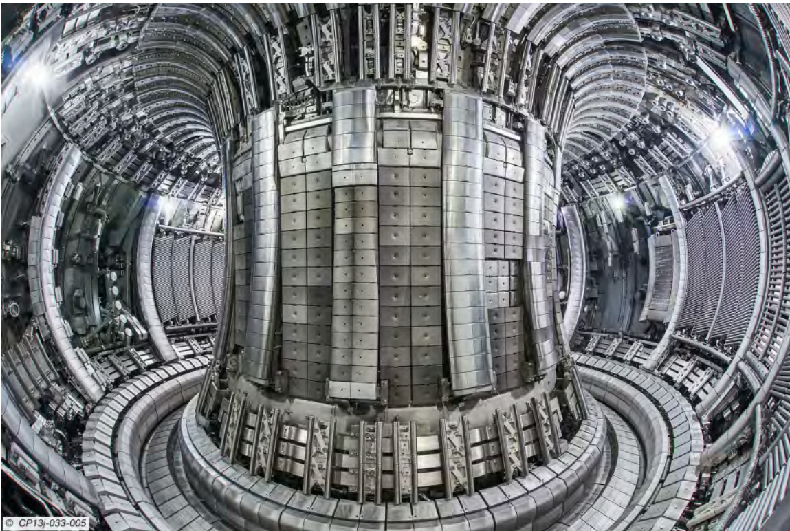
Figure 10.25 The Joint European Torus (JET) tokamak fusion detector uses magnetic fields to fuse deuterium and tritium nuclei (credit: EUROfusion).
