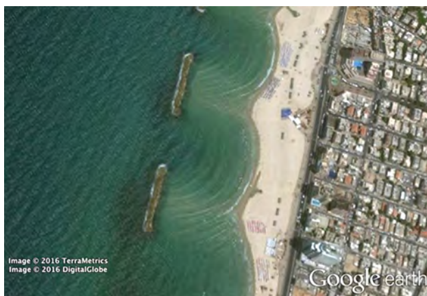
Figure 4.2 Because of the diffraction of waves, ocean waves entering through an opening in a breakwater can spread throughout the bay. (credit: modification of map data from Google Earth)
