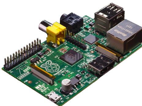
**Figura 19** – *Raspberry Pi* Modelo B
