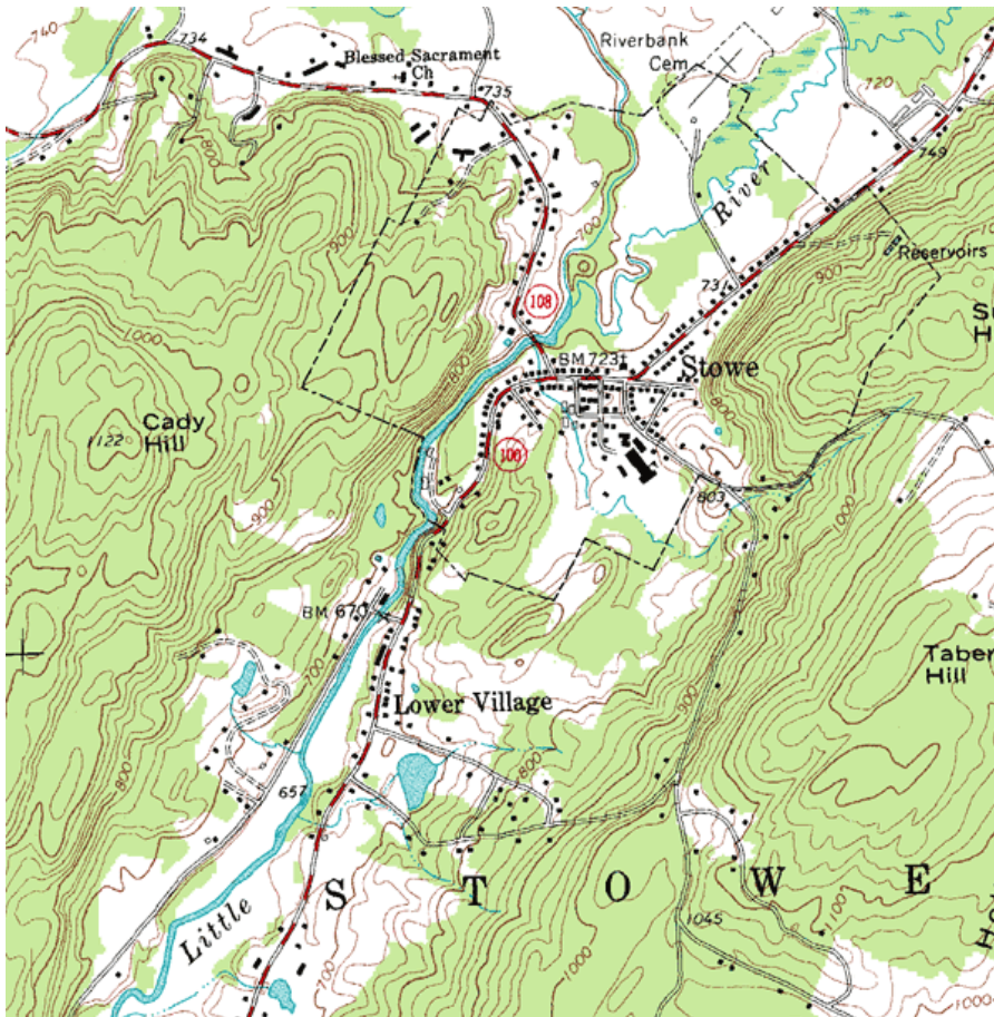
Figure 2.29: Portion of a USGS topographic map of Stowe, VT. In this map, you can see how the spacings of the contour lines indicate a steep hill just to the right of the city of Stowe in the right half. The hill becomes less steep as you proceed right.
