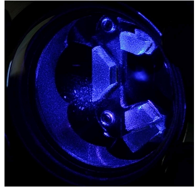
Figure 24.9: Picture of a strontium MOT operated at 461 nm. The atomic cloud, which consists of about 10^6 atoms at 10 mK temperature is visible as a diffuse spot located inside a three-mirror ring cavity (courtesy: Camila Beli and Michelle Moreno).
