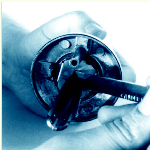
FIGURE 43 —Insert the forked end of the cylinder removing tool into the lockset as shown.
