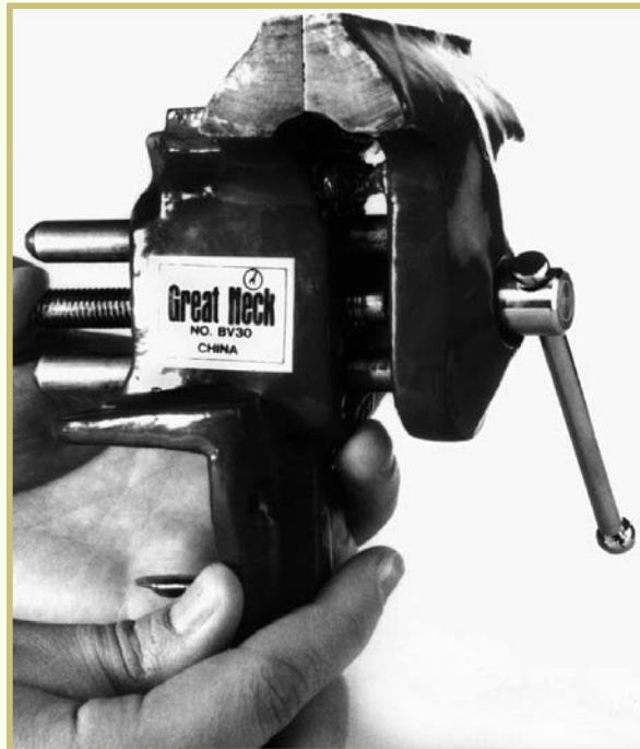
FIGURE 1—A quality vise will help you hold keys, plugs, and lock shells tightly while working on them.
