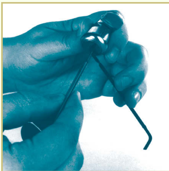
FIGURE 8—Hold the tension wrench and the pick as shown here when picking a lock.
