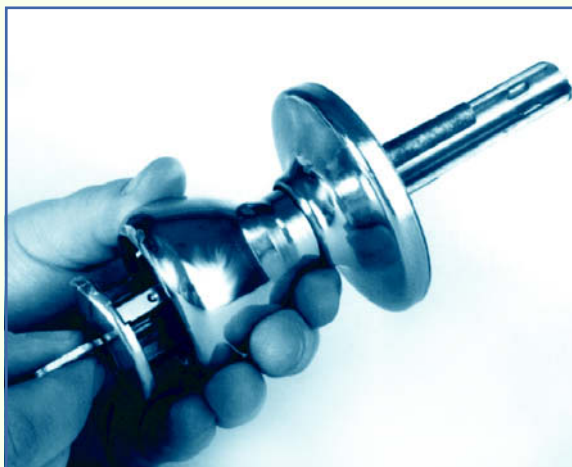
FIGURE 45—The cylinder should pop out into your hand.
