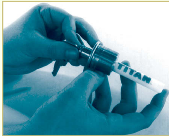
FIGURE J—Use a plug follower to push the plug out of the cylinder.
