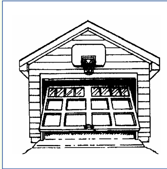
FIGURE 8—Overhead Garage Door
