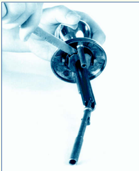
FIGURE 42 —Turn the lockset over, and the spindle will fall out.
