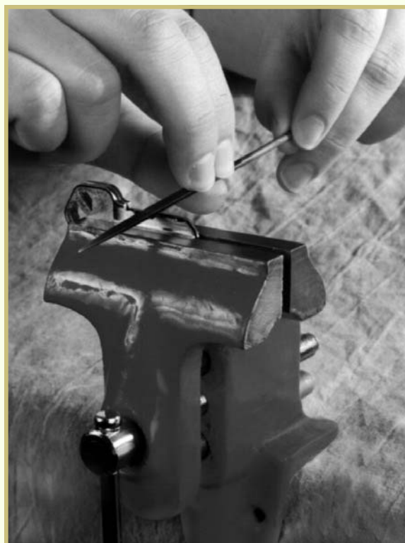
FIGURE 13—This is the proper way to hold a file to make clean, square cuts in the blank key.
