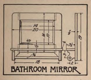
out the back edges around the opening to hold the glass. The vertical pieces, it will be noted, extend downward to hold the shelf-brackets, which may now be made ready. If a roller-towel is to be used, one bracket must have a hole clear through, so that the roller may be withdrawn. It then remains only to make the shelf and assemble the parts. Glue the mortises; fasten the other pieces with screws from behind, and glue.
