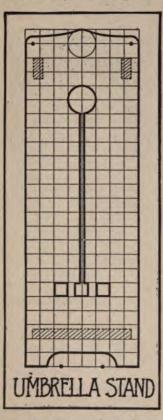
fectly square and flat on the ends. Mark off on the inner surface of each side board just where the other pieces are to be fastened. Fasten one of the sides to the bottom, and then nail on the cross pieces, after which turn over and put on the other side.
