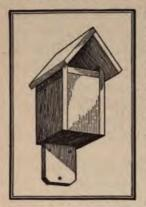
cover the ridge with a strip of zinc or tin to shed the water. It is a good plan in sawing out the entrance to make the outside diameter somewhat larger than the inside, as this will tend to keep the water from trickling inside during a driving rain.
