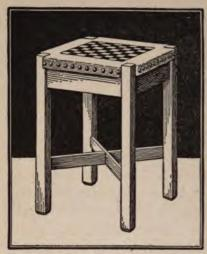
The four identical upper crosspieces are now in order, and will be tenoned to match the legs, after which the eight pieces thus far made will be fitted together so that the exact length of the diagonals may be determined. These latter will then be made ready, and each must be notched out, where they cross in the center, to one half its depth.
