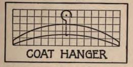
enough for us to mark out three rows of oneinch squares, fifteen squares to the row. Tack this down and then tie a piece of string to a lead pencil in order to draw the two curves, which is a very easy matter when the other end of the string is tied or looped around a tack. For the top curve the
