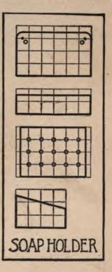
which the four pieces may be nailed together, using two or three small wire nails for each connection. The bottom is now to be sawn out just large enough to fit inside. Bore a number of quarter-inch holes in this, as shown in the working drawing, and then nail in place.
