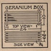
the bottom, and it is a simple matter to add a pair of sides and then a pair of ends until they are all in place. Use the square to make sure that the sides and ends are going up squarely, and always nail in at an angle so that the nails of the next pair of strips will not interfere.
