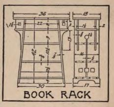
tire outline, positions of the shelves, dowel-pin holes, and the ornamental openings, then proceed to work carefully down to these lines, having in mind all the while the necessity of obtaining a good clear outline at whatever angle the piece is viewed.
