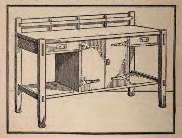
end. The rear legs are similar to the front ones in every way, except that they extend above the top board to hold the plate-rack. Having completed the legs, the two crosspieces of each end should be planed up and then tenoned to fit the mortises already made in the legs. The pieces thus far made should now be put together with glue and firmly clamped until set, taking due care to have the several
