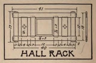
their respective mortises, after which the entire frame may be assembled. Use glue at all connections and clamp firmly until thoroughly dry. The mirror is held in place by notching out the back edges of the four pieces that surround it, so that it can be set in from the rear.
