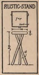
method will be obvious when the crooked pieces are all arranged in place. Around the four edges of the top are nailed pieces sawed from the sides of a small branch with the bark in place. The top should be given at least one coat of oil to protect it from the weather.
