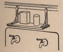
and a board on top, and the job is done. But supposing there is no room for brackets, as, for example, is usually the case over the kitchen sink, what then? Just turn the brackets upside down and "hang" the shelf in place. If the place where
