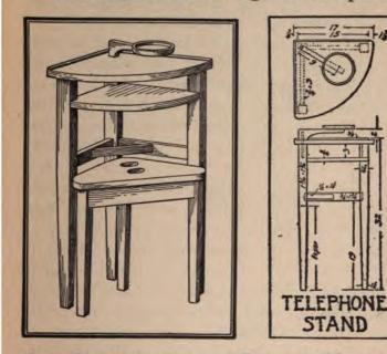
about the same as for a small square table, except that one leg is missing. First square up to length the material for the three legs, and after marking out the mortises and guide-lines for the tapering portions work them carefully down to line. The several crosspieces will now be cut to length and tenoned to match the legs. The whole should now
