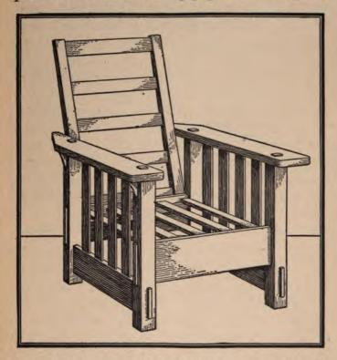
the back is easily adjusted by moving two looselyfitting pegs, which are set into holes bored in the rearward projecting ends of the arm-rests.
