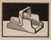
From any machinery or arts-and-crafts supply house strips of brass or copper may be obtained very reasonably. A pair of tin snips and a file will do all the shaping, and the punch-
