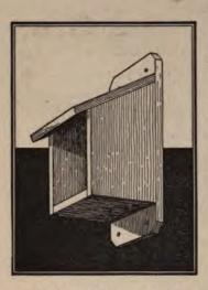
prefer to nest under the eaves, and require nothing more than a little nook or corner. The accompanying sketches illustrate a suitable form of nesting shelf, the construction of which is very simple. If several of these are to be put up, make one or more with one side open as well as the front.
