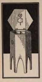
any difficulty is contemplated in assembling make a second hexagon to act as a temporary top. This latter will keep the side in pieces their relation proper while they are being fastened to the bottom and glued along the edges. Before assembling,
