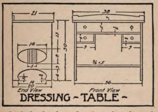
snugly fit in the three slats in each end opening, securing each slat with glue and a wire nail at each end. It now only remains to make and fit the drawers—and our table is complete.
