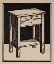
sure that nothing is on the floor to mar it.) Fasten each leg to the top with glue and three long screws set in at an angle. With very fine sand-paper go over the table and slightly remove the When corners. sand-papering the top and legs do not hold the paper in
