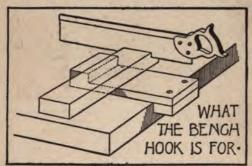
one must have what is called a bench hook. The way it is used is clearly illustrated, but its full advantage cannot be appre-
