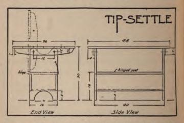
front and back edge of each end board should be notched to a depth of one inch, in order that the front and back boards may be set in flush. After boring two three-fourths-inch holes for the hinge pegs, the ends may be set aside. The front and back boards next demand our attention. These require nothing further than trimming up square and to the proper dimensions. The end boards may
