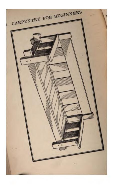
round the ends slightly. Prepare the two crossbars, making the ends perfectly flat and square. Towards the lower end of each of the four corner posts a section is cut out so that the long runners will set in half an inch, as shown in the end drawing. view Mortises, three-fourths of an inch wide and one and one-quarter inches deep, should then be cut for the back rail.
