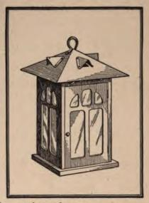
ing four triangular covered openings in the top, which is to be made of galvanized iron or of heavy tin, painted a dull black.
