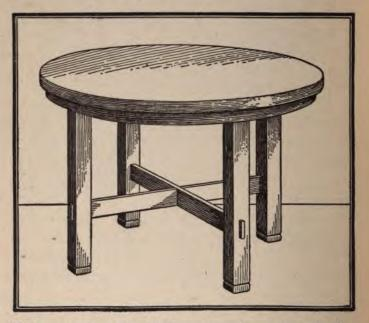
If the amateur has had no experience in this line, it is best to have the lumber-mill do it for him. Secure good clear lumber of fair width and, after truing up the edges, lay the several pieces on the bench and draw a circle about an inch larger than the finished top. Rough out the boards with the saw, and join them with fresh glue, clamping
