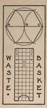
full circle through A and C. Join up the points where the circles cut each other and you will have a perfect six-sided figure, which, by the way, is called a hexagon. Remember you do not have to change the compasses once after they are properly set.
