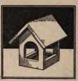
covering the ridge with a strip of zinc or tin. A small strip of wood should then be nailed on along each of the two sides to hold the nesting material in position.
