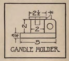
and in sawing this out be sure to get it perfectly square and flat on the ends or there will be seams at the top and bottom when the other pieces are put on. Bore a hole in the center the size of a candle and three-quarters of an inch deep and then fasten the block in the exact center of the base board and square with the sides by nailing up through the bottom. The top piece is now to be marked out and the exact center found by drawing
