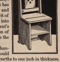
measure from three-fourths to one inch in thickness. First, work out the two side-boards of each side, and see to it that when they are placed together they will form the proper shape for the side of the chair. Set the two front halves aside, and proceed to construct the entire back half of the chair. Prepare the rear portion of the seat-board and then the crosspiece that sets on the floor at the rear. The two sides may now be set up and connected, using glue and screws at all connections.
