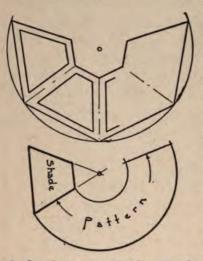
pattern: on a large sheet of paper draw out the shade and then continue the slanting side lines up to an intersection; with this point as a center draw a large and a small circle as shown, after which it only remains to step off a distance along the larger arc equal to the circumference
