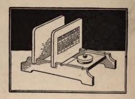
the compasses and then cut the wood exactly to line. The upright pieces are set into slots cut in the sides, so be sure that these slots are just large enough to make a tight fit. After the two sides are cut to line, place them together, sandpaper the edges flat and smooth, and hollow out the places for the pen and pencil. The two upright pieces require no attention aside from having their ends made smooth and the corners rounded. The last of the five pieces is for the ink pot, and should
