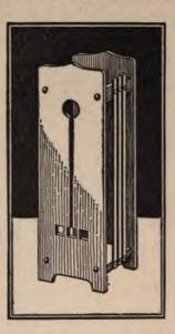
with the fret saw, which should also be used for the circular opening near the top. The long, narrow slot may be worked out with the knife, although sawing will be the safer way. See that all edges and corners are finished sharp and true, and then shape up the top and the two feet at the bottom.
