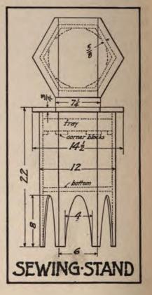
fit everything together, and provide means for clamping while the glue sets. To strengthen the side seams and to act as a support for the tray, make six little blocks as shown in the working drawing, and fasten them in place with glue and screws. The tray may be made as deep and in as many compartments as desired. The top is more apt to retain its shape if made of three pieces, fastened with glued tongue-and-groove connections.
