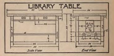
inch boards, reënforced around the edges with a narrow board, to give it a massive appearance. The top was then covered with a dark shade of imitation leather, fastened with large-head, dullfinished brass nails.
