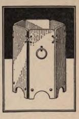
mark one board from another, but use the compasses on each one separately. Six quarter-inch holes must now be bored in each piece as indicated, due care being taken not to tear off any splinters.
