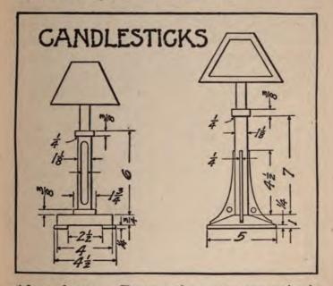
with sandpaper. Prepare the center post as in the previous case except that the sides are left plain. Make ready the four curved brackets, and in finishing their edges work up all four together so as to avoid rounding. Now fit together the whole, and after marking off the position of the brackets on
