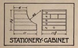
small brads. The entire structure should be assembled before making the drawer, which, with the exception of the front, should be made from as thin material as possible.
