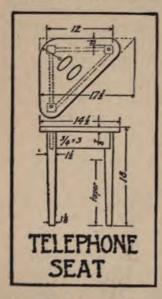
may be made fast with glue and a wire nail or peg through each mortise and tenon.
