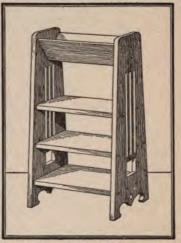
ings, the positions of the shelves and the dowel pins. After removing the surplus material, a hole should be bored at the end of each slot and in each corner
