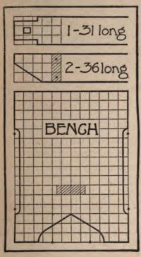
The material is all one-inch dressed lumber. The working drawing clearly shows how to mark out the end pieces. By examining this you will find that you will have to make six different curves with the compasses. This, however, is a very simple matter as the sizes and center points are all indicated on the drawing, and as soon as the curves are drawn it is only necessary to
