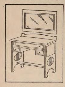
foot-rail are to be trimmed up to their respective widths and to the same length. As soon as the top has been made ready, the two sides are to be set up and connected. On account of the direction of the grain in that portion of each side just below the elliptical openings,
