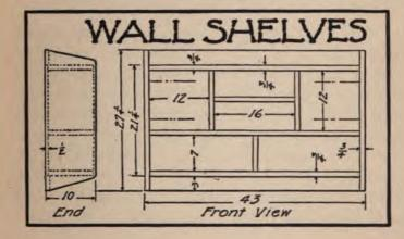
should be nailed in place. The connections of the upper two shelves may be made by means of small blocks glued and nailed in the corners of the two compartments. Use glue on all joints.
