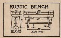
on the underside near each end to receive the supports, the latter should be taken up. Mark out the outline and positions of the mor-
