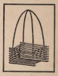
construction, nail four of the larger sticks together, so as to make a frame with the ends projecting about one and a half to two inches. Between the two upper sticks place a row of sticks so as to form a grating with half-inch spaces. This makes the
