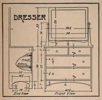
top board. The back should now be closed and the curved foot strip shaped up and secured in place, after which the drawers will receive our attention. A moment's inspection of any well-made piece of furniture will clearly indicate the best and most workmanlike manner of connecting the several thin
