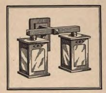
With the present design a simple method of connecting shades to ordinary key sockets is introduced that will undoubtedly appeal to the amateur craftsman. A hole is cut in the top of
