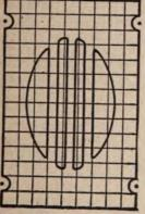
remains to make two slots in the two upper crosspieces to receive the ends of this piece, and the whole chair may be assembled. Set up with glue, secure each joint with a small peg or wire nail, and clamp until set. Small square strips should be attached to the inner surfaces of the four seat crosspieces, after which the seat-
