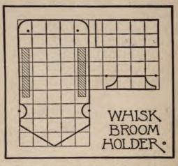
rub the edges smooth with a piece of sandpaper wrapped on something round that will fit the curves. Before nailing up, hold the pieces together and put in the broom to make sure that it will fit. If it is very large or very small, some change may be necessary. Fasten the sides on by small brads driven in from behind, and while the front may also be nailed on, a neater appearance will result if it is fastened with glue and put under a heavy weight
