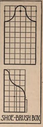
the front, after which the bottom should be cut so that it will fit snugly inside. Nail this in place, and then fit in the center piece, which is fastened in place by nailing in through the sides.
