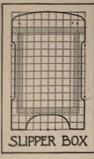
carefully so as not to tear off any splinters, and then take the plane and knife and trim down to line. Test the edges frequently, or you will be sure to trim off more toward one side than toward the other. When the two are finally shaped up, place them together, and sandpaper the edges smooth with 8 piece of sandpaper
