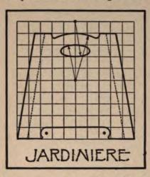
reduced by the thickness of the other two sides, otherwise our box will not be square when we look down upon it. Set the heads of the nails deeply. Apply a coat of linseed oil inside and out, and when this is dry putty up the
