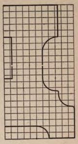
The panels are of threeeighths-inch board, in which is cut the mission cross. These panels should be mortised above and below into the crosspieces for a distance of about one-fourth of an inch. The entire
