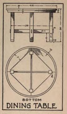
angles with the top. Next attend to the legs. In forming the feet make a saw cut on the four sides to a depth of three eighths of an inch, and then finish with the chisel. Mark out the position of the mortises for the tie pieces, and cut them from both sides. Carefully determine the length of these tie pieces and tenon them to match the legs. When the tie bars pass one another at the center, cut down each one to half its width. Put the legs and tie
