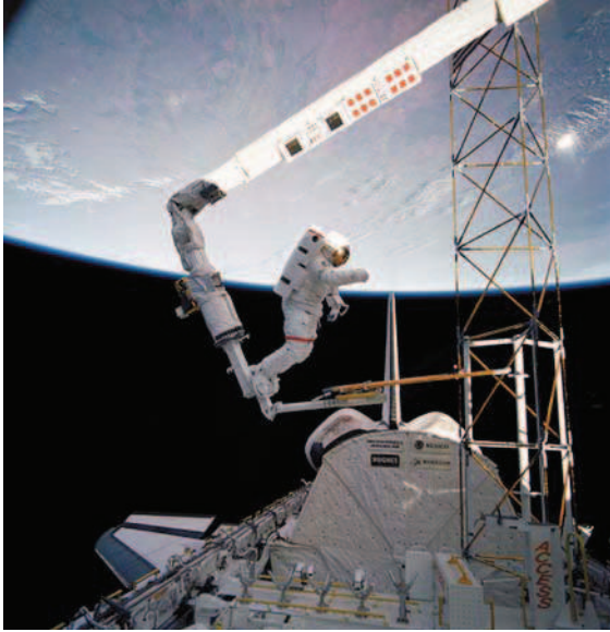
Fig. 45.3 Space shuttle remote manipulator system (SRMS) used as a platform for an astronaut's extravehicular activity in the shuttle cargo bay
