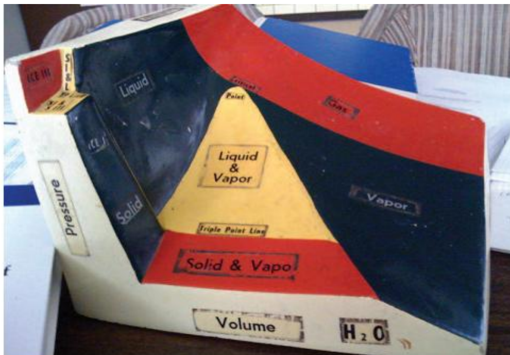
Figure 3.22: P - v - T surface for H_2O , showing solid, liquid, and vapor phases.
