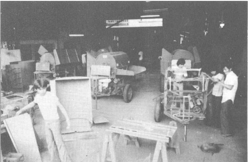
12. Axial-flow thresher Model TH3 production by a medium-size firm (M/s Kaunlaran Industries, San Pablo) in the Philippines.
