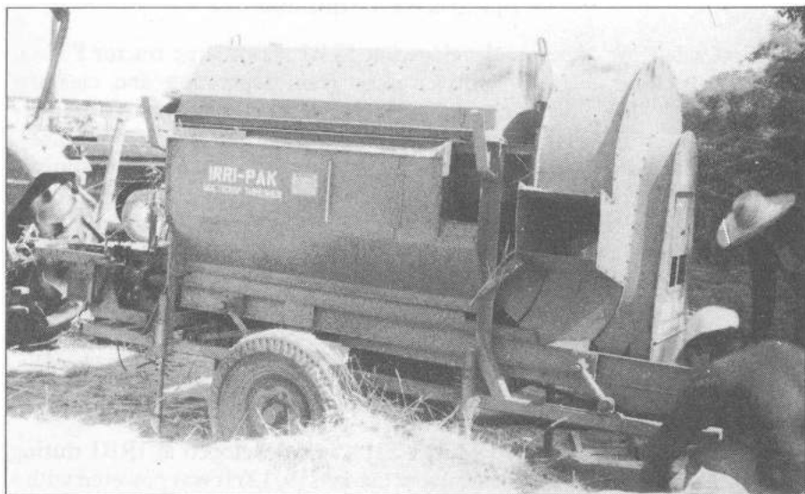
6. Tractor PTO-powered, axial-flow thresher, Model IRRI-PARC-30 being used for threshing paddy in Pakistan.
