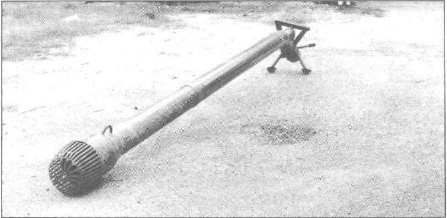
7. Present design of the axial-flow pump in the Suphanburi area, Thailand.
