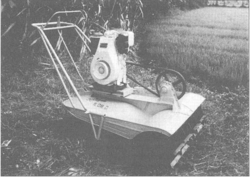
1. Turtle power tiller (MSF model) with 14 hp air-cooled diesel engine.
