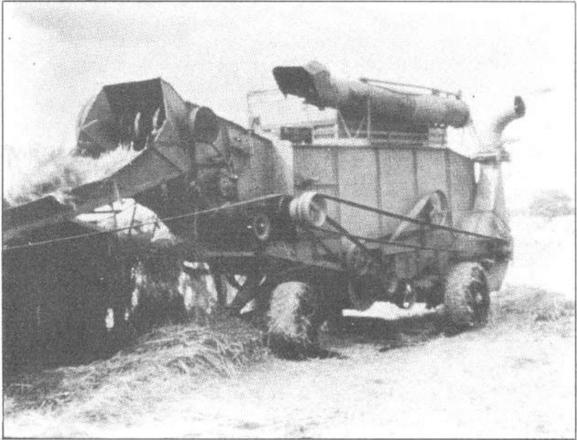
3. McCormick-type (tilladora) thresher used in Central Luzon for custom threshing of paddy.
