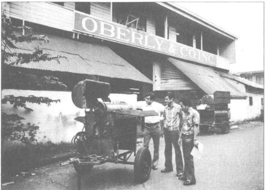
11. Axial-flow thresher with an oscillating screen manufactured by Oberly & Co., Inc.
