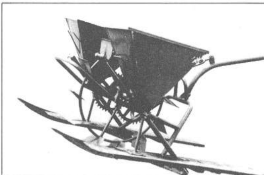
2. Combined underground and surface closure for minimizing N transfer to floodwater during deep placement.
