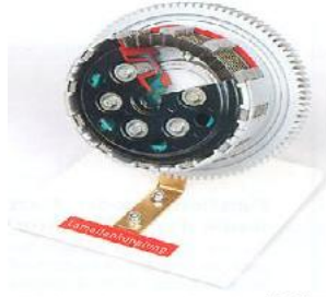
Fig: Cutaway Model Of Multi-Plate Clutch
