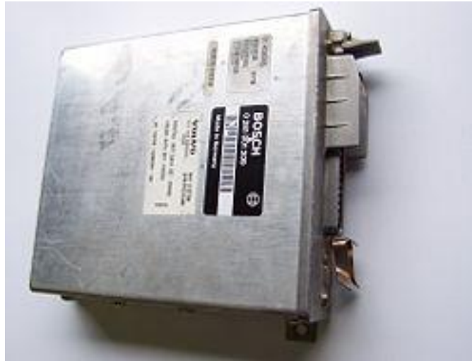
EDC control unit
