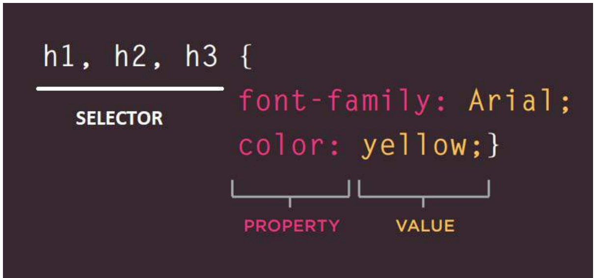
Figure 5: CSS Selector using multiple HTML elements
