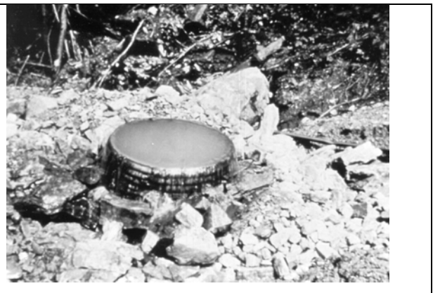
Figure 10.5b. COE stilling well.
