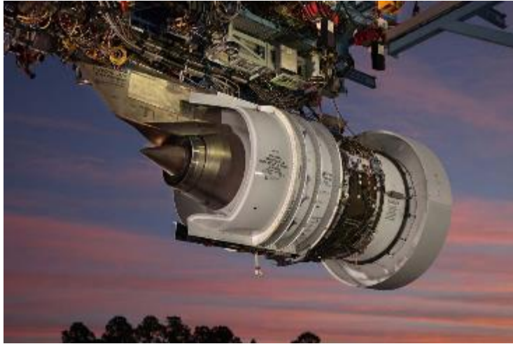
PW1100G on test
