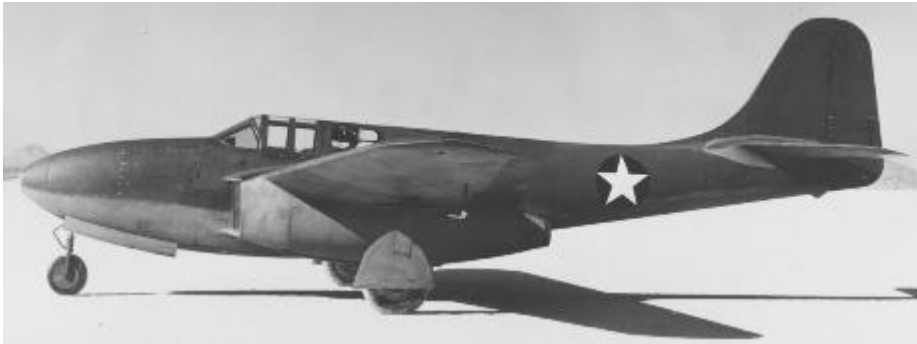
The Bell XP-59A Airacomet first flew on 1 October 1942, powered by two GE I-A engines.
