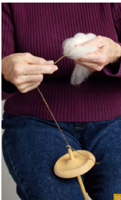
(10) With one hand, hold a handful of fiber and the leader together.
