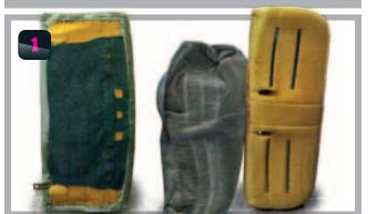
Remove seats from the vehicle and place all bolts and other fasteners into a marked container. Then, using pliers cut the hog rings using generally located on the edges of the rear side of the seat. Also, unclip any plastic retaining hooks and detach
