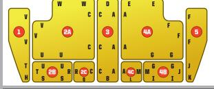
Using a marker label on the back of the material. Here we are simply using a simple 1-9 pattern labeling each seat portion and A-Z for labeling adjacent sides. (You can choose your own system; just make sure it is consistent and accurate. It may also help to sketch out a picture or diagram of the seat.)
