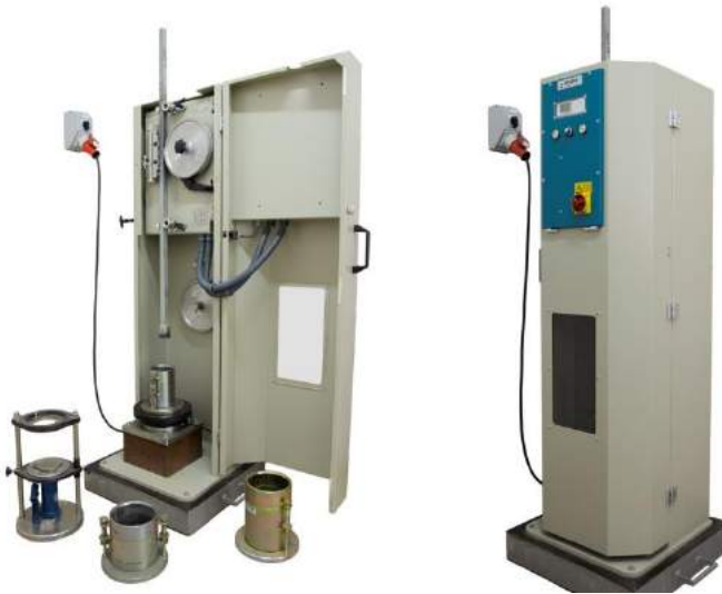
Fig. 1.12. Proctor's device used in geotechnical laboratory (Faculty of Civil Engineering at Warsaw University of Technology).
