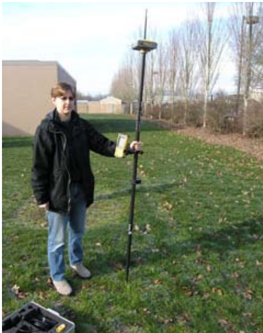
Figure 1-80 Typical setup for the base station over a known control point. The operator has used the optical plummet to center the base. Once the base is set, careful vertical measurement of the antenna slant height is made.
