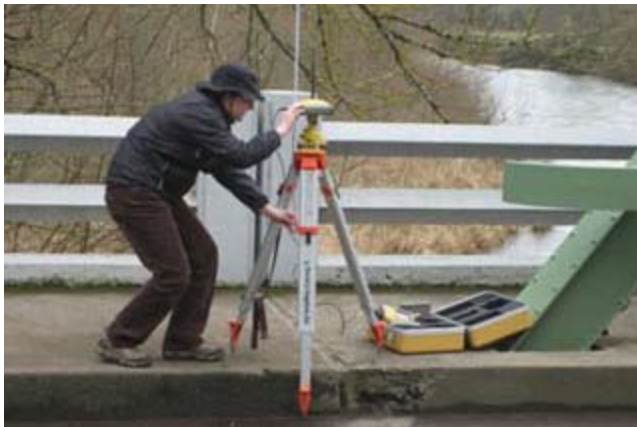
Figure 1-80 Typical setup for the base station over a known control point. The operator has used the optical plummet to center the base. Once the base is set, careful vertical measurement of the antenna slant height is made.
