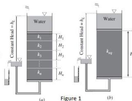
Figure 1b shows an “equivalent” soil layer that can replace the stratified system shown in Figure 1a.
