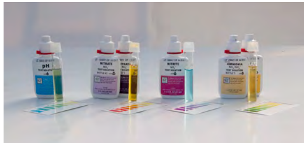
Fig. 5.7 Ammonia Test Kit Showing a Small Increase in Ammonia Levels (0.25-0.5 mg.l)
