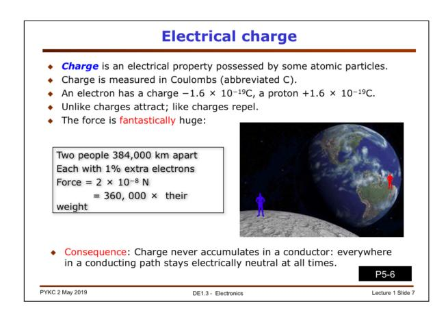
The foundation of electronics is of course the electrons you found inside atoms. Each electron has electrical charge, which is measured in Coulombs (C). An electron's charge is negative, and is measured as  $-1.6 \times 10^{19}$  C, which is pretty small. This is balanced out by the proton in the atom, which has a positive charge of  $+16 \times 10^{19}$  C.
