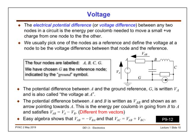
**Voltage** is the electrical **potential difference** between any two nodes in a circuit. It is the energy required to move 1 Coulomb of positive change charge between the two nodes.
