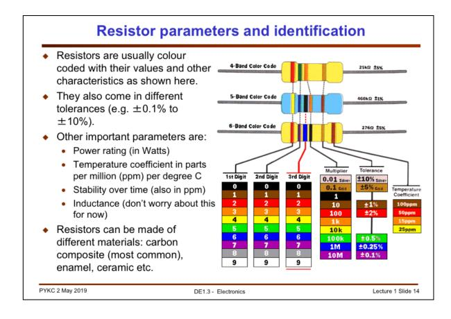
A resistor is characterised by a number of parameters:
