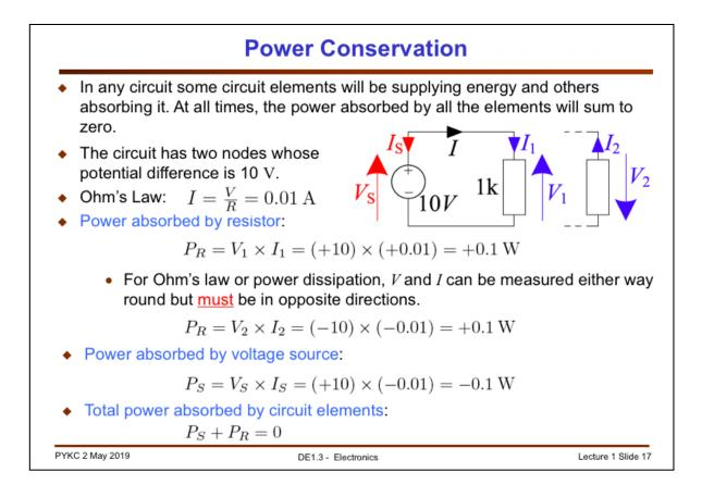
The law of conservation of energy (hence power) applies in electronic circuits. Consider the simple circuit above. Power absorbed by the 1k resistor connected to a 10v battery is 0.1W. If you reverse the voltage ( $V_2$ ) the current ( $I_2$ ) must flow from high voltage to low voltage, and therefore is reversed (i.e. pointing up). Using this second convention, the power is still 0.1W.
