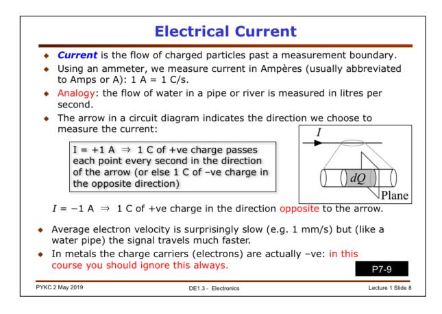
Electrical circuits would not be doing anything useful unless current flows in them. Electrical current is the flow of charge (electrons) as measure at a certain cross section. This is really similar to water molecules flowing through a pipe.
