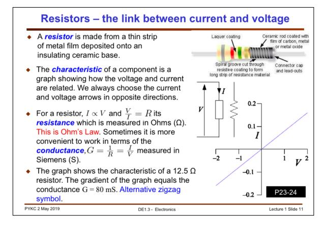
The most basic component in electronics is the resistor. Its value, the resistance R provides the simple relationship between voltage and current through Ohm's law.
