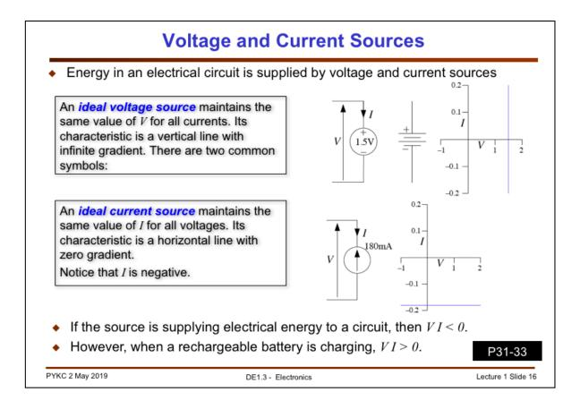
There are two other common components: 1) an ideal voltage source that has a constant voltage value no matter how much current are flowing from it; 2) an ideal current source that can provide the fixed amount of current no matter what the voltage is across the source.
