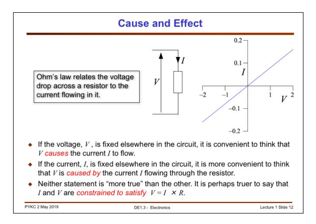
Resistor is said to be a "linear" component, because the current vs voltage characteristic is a linear function (i.e. straight line). The gradient of the line is the conductance.
