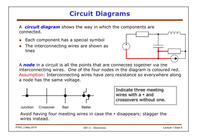
We often represent electronic circuits in the form of circuit schematic in a diagram form. Here is a circuit with components connected together. The lines connecting the components together are called "Nodes". In this circuit, we have four notes. The one shown in red is quite large, but we assume that no matter where you are on this red node, you will have the same electrical voltage. In other words, the wires associated with this node is assumed to have zero resistance.
