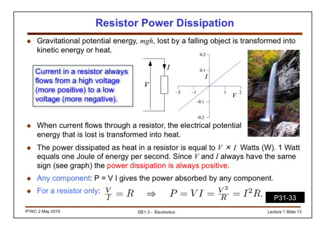
Whenever current flows through a resistor, energy is dissipated as heat. This is analogous to falling by a distance and converting the lost potential energy into kinetic energy.
