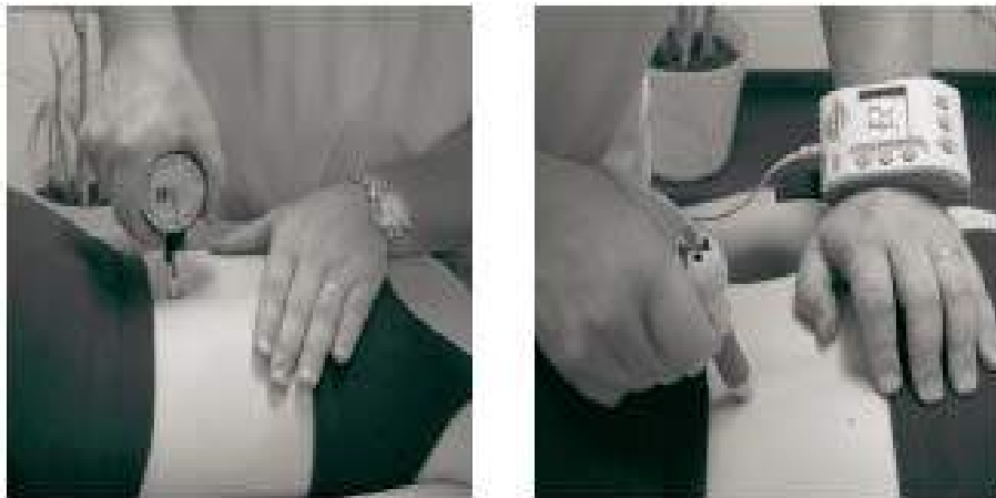
Figure 3. Hand-held algometer (Neuromechanical Innovations, Phoenix, AZ) (Left) and Commander PainTrack™ (J-Tech Medical Industries, Salt Lake City, UT) (Right) being administered to the lumbar spine
