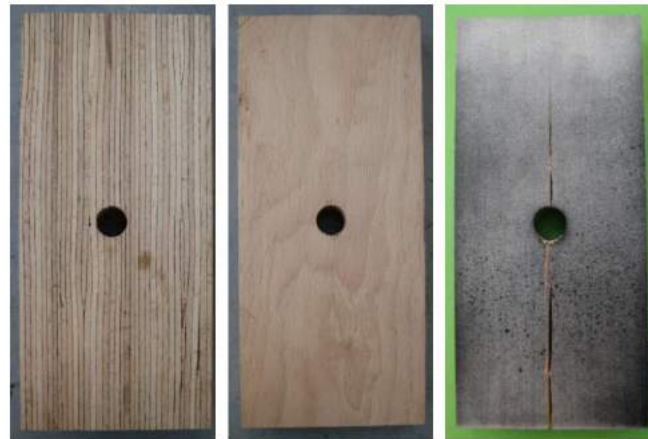
Figure 9. Beech LVL specimens for embedment tests with edgewise-arranged veneers (left), with flatwise-arranged veneers (centre) and with stochastic pattern after testing (right) [34].
