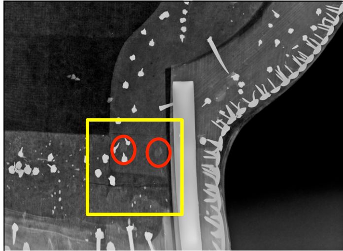
Fig. 37: X-ray illustration of joints
