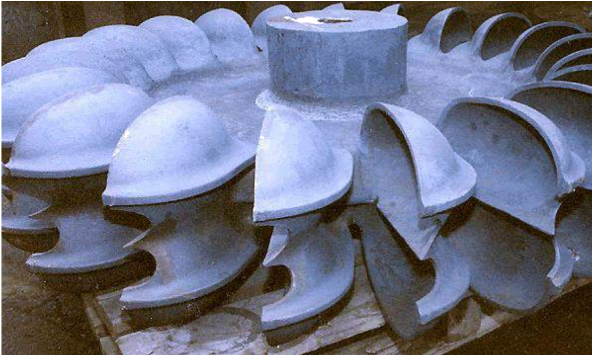
Figure 26.1 Typical PELTON WHEEL with 21 Buckets
