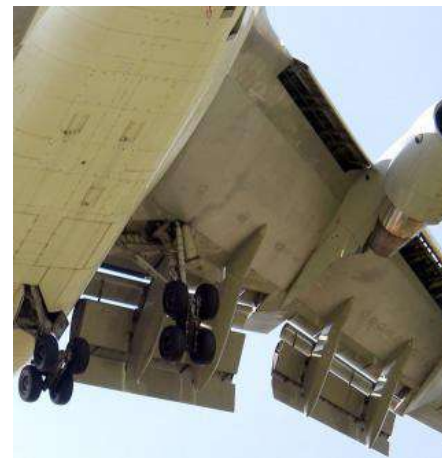
multi-element trailing-edge flaps
