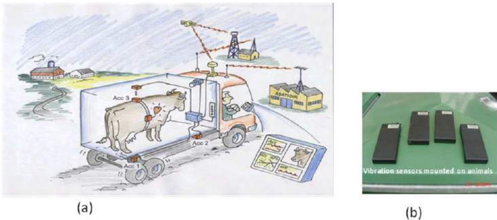
Fig. 3. (a) Sketch of instrumented vehicle showing the positions of sensors , video camera and GPS; (b) vibration sensors mounted on animals
