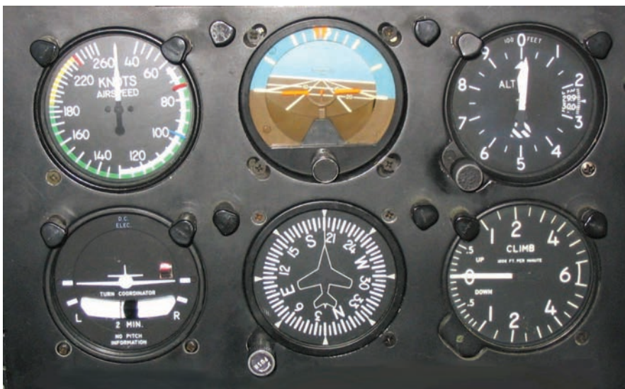
Figure 5.8: Six basic instruments in a light twin-engine airplane arranged in a basic-T . From top left: airspeed indicator, attitude indicator, altimeter, turn coordinator, heading indicator, and vertical speed indicator. © User:Meggarr / Wikimedia Commons / CC-BY-SA-3.0 .
