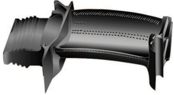
(b) A schematic of a high-pressure turbine blade as used in aircraft jet engines. © User:Tomeasy / Wikimedia Commons / CC-BY-SA-3.0.
