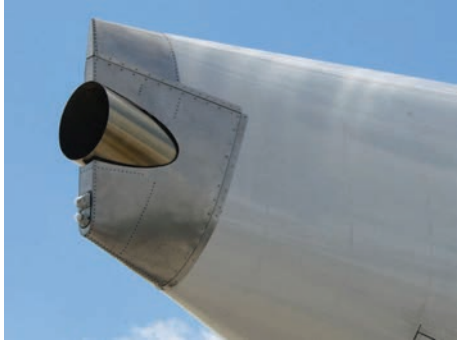
(b) The APU exhaust at the tail end of an Airbus A380. © David Monniaux / Wikimedia Commons / CC-BY-SA-3.0.
