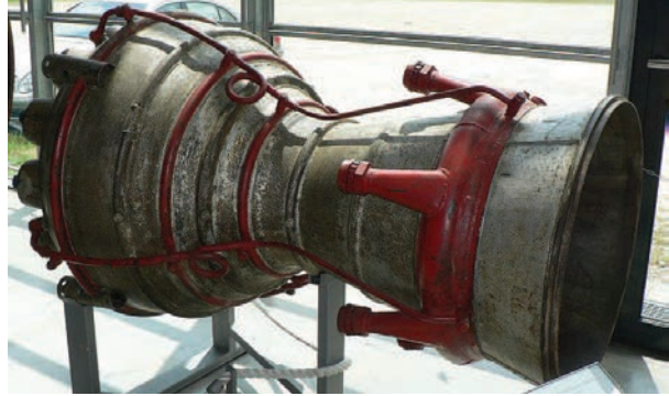
(a) Convergent-divergent nozzle diagram. User:OK / Wikimedia Commons / Public Domain. (b) Convergent-divergent rocket nozzle. © User:Jaypee / Wikimedia Commons / CC-BY-SA-3.0.
