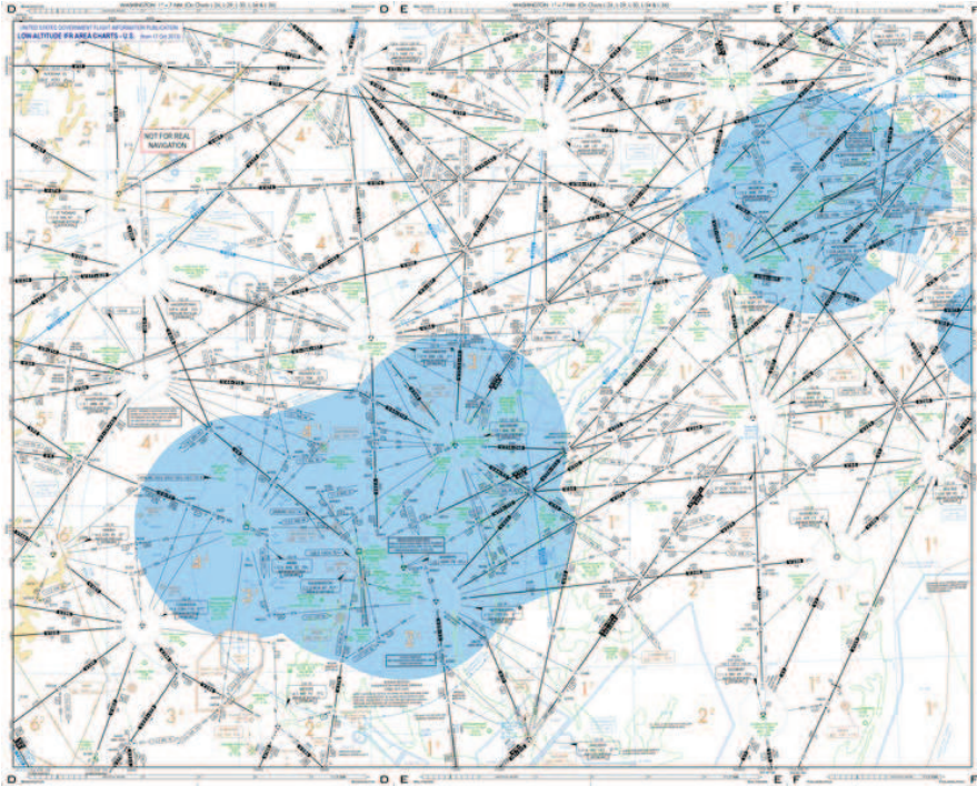
Figure 10.9: This low altitude section chart is issued for use in air navigation under IFR. The dimensions of this depicted area around Washington D.C. are nearly 280 and 220 nautical miles. Author: User:Orion 8 / Wikimedia Commons / Public Domain.
