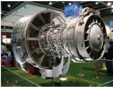
(c) Turbofan CFM56 (high by-pass). © David Monniaux / Wikimedia Commons / CC-BY-SA-3.0 .
