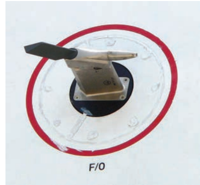
(a) Diagram of en:pitot-static system, including static port and pitot tube as well as the pitot static instruments. Author User:Giggy. / Wikimedia Commons / Public Domain. (b) A380 Pitot tube. © David Monniaux / Wikimedia Commons / CC-BY-SA-3.0 .
