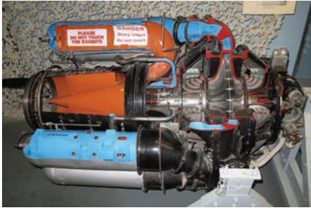
(a) A Rolls-Royce Welland jet engine cut away showing a centrifugal compressor. © user:geni / Wikimedia Commons / CC-BY-SA-3.0.
