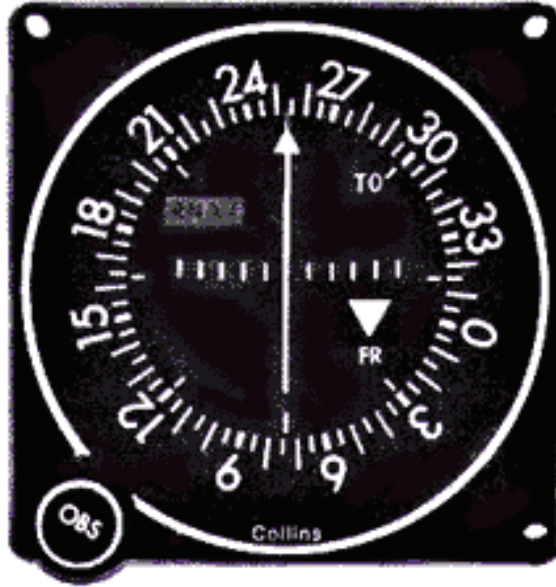
(a) Onmi-Bearing Indicator: the VOR intercepts the aircraft in radial 250 (approx.); the CDI (white vertical bar) indicates that the aircraft is flying in the direction of the radial; The To-From indicator (indicating From) says that the aircraft has already overflowed the VOR station and keeps going. Author: User:Quistnix / Wikimedia Commons / Public Domain.
