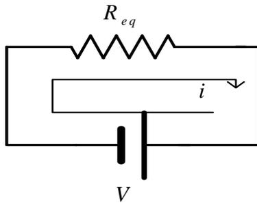
Donde  $R_{eq} = R_1 + R_2 + R_3$
