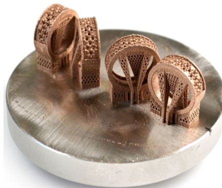
Figure 2.6 – Sample of finished products on the plate just released from SLM printing
