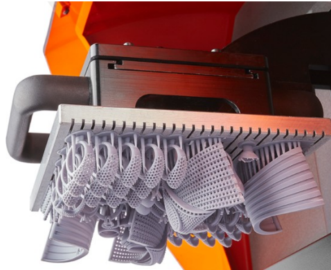
Figure 2.5 – Palette with newly printed jewelry with the SLA technology
