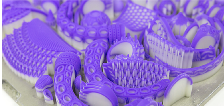
Figure 2.7 – Samples of wax printed jewels (the purple wax is the jewel itself and the white one is the support)
