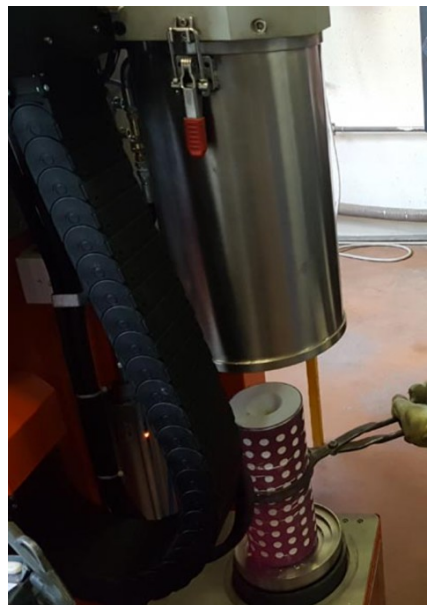
Figure 2.4 – Metal casting machinery in the cylinder emptied of wax
