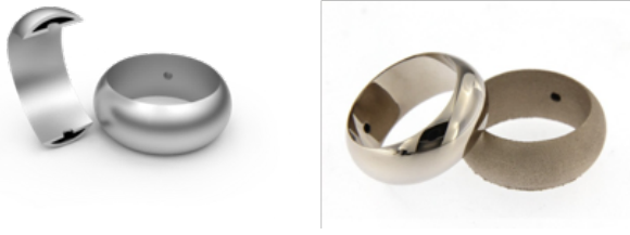
Figure 5.1 – Example of hollow faith made by SLM with a small hole (3D model on the left and printed object on the right) Source: see [28]
