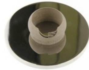
Figure 5.2 – White gold ring with hollow inside, cross-section with and without reticular support structure. Source: see [28]
