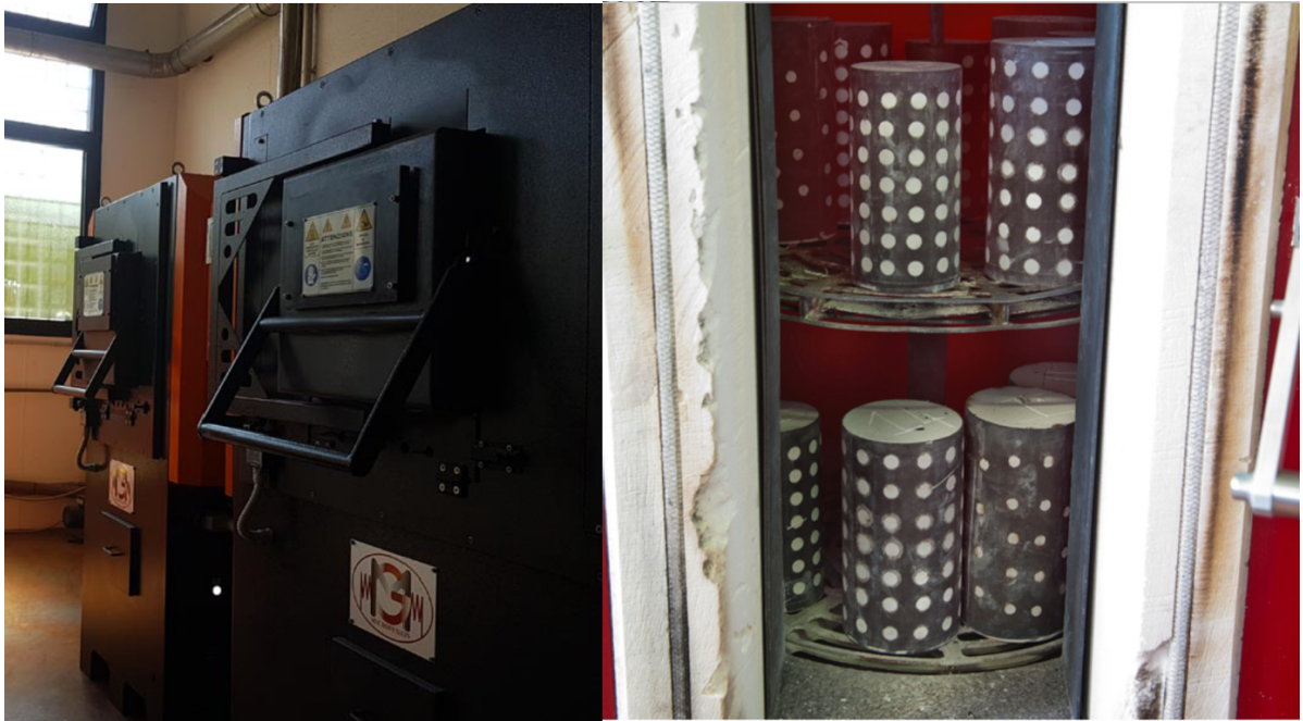
Figure 2.3 – Cylinder baking machinery for wax leakage and cylinders inside the machinery
