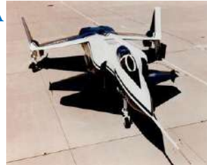
Fig. 20.4 Conventional engine, no lift engines, flow diversion used.
