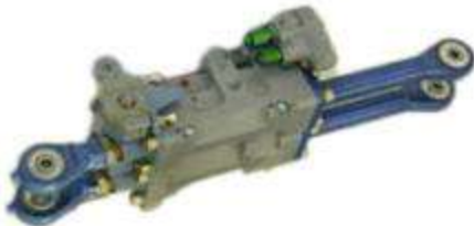
(a) Mechanically-signaled/hydraulically-supplied duplex-parallel aileron actuator for Dassault Falcon 900 private jet
