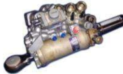
(b) Electrically-signaled, hydraulically-supplied (HSA) simplex actuator for rudder actuation of Boeing B777
