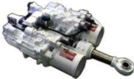
(d) Electrically-signaled and supplied EHA for the JSF F-35 fighter
