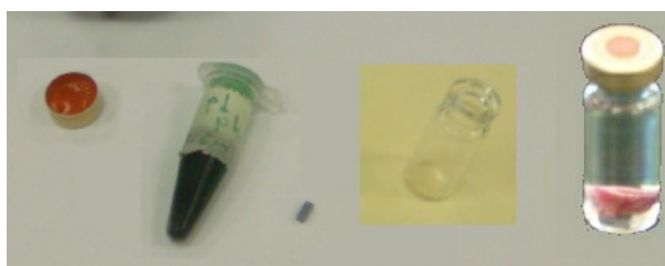
Fig. 2. A sealed reaction vial containing Pd phosphor solution, stirring bar and a mouse liver specimen.
