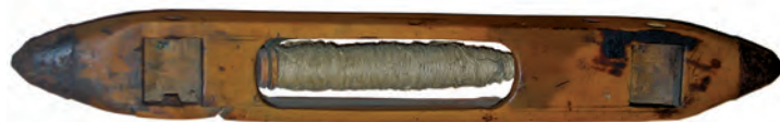
Source 5.41 The flying shuttle allowed the thread to be shot back and forth across a wider weaving bed, producing much wider lengths of cloth, much faster.
