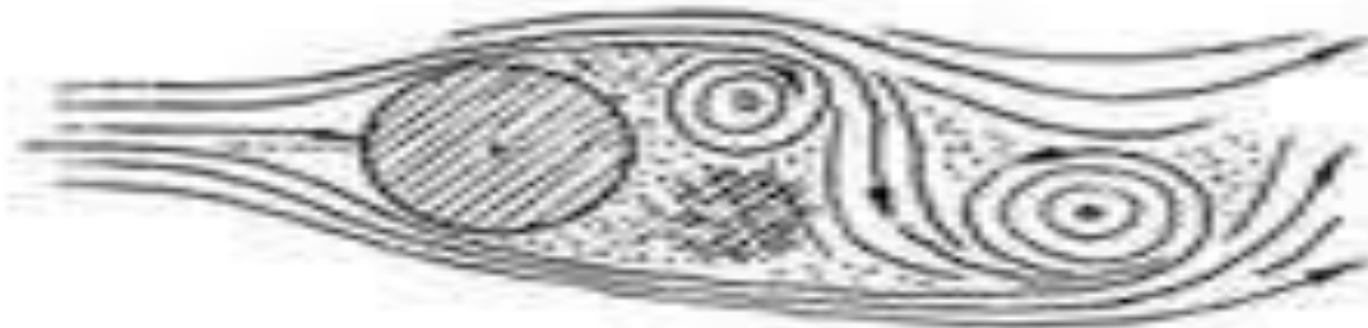
(c) CYLINDER BETWEEN Re = 10^2 AND 10^3 ; VORTEX STREET WITH C_{D_{max}} = 1-2
