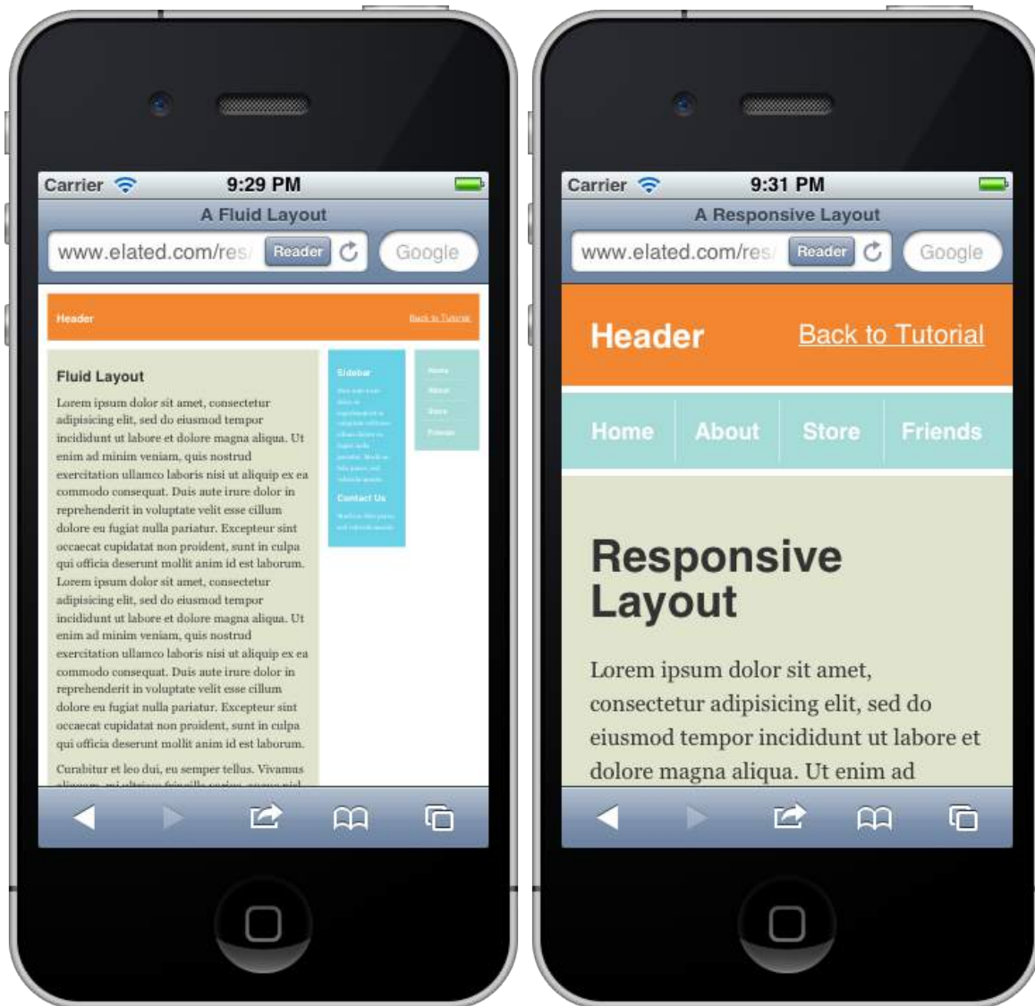
Figure 3.3: On the left: viewing a desktop website in Mobile Safari on iPhone. Not a fun experience. On the right: viewing a mobile optimized website in Mobile Safari on iPhone.
