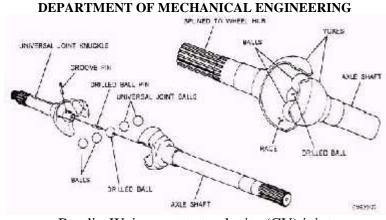
Bendix-Weiss constant velocity (CV) joint
