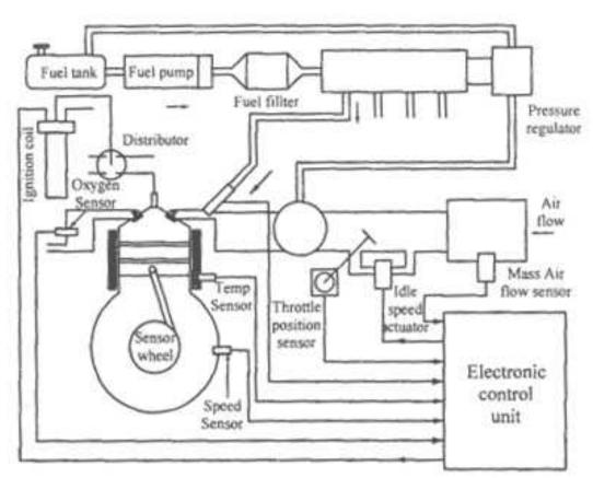
Engine management system with sensors and actuators
