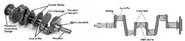
The parts of the crankshaft inside the main bearing are called main journals.
