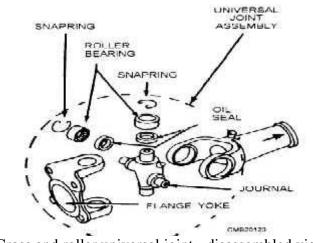
Cross and roller universal joint - disassembled view.
