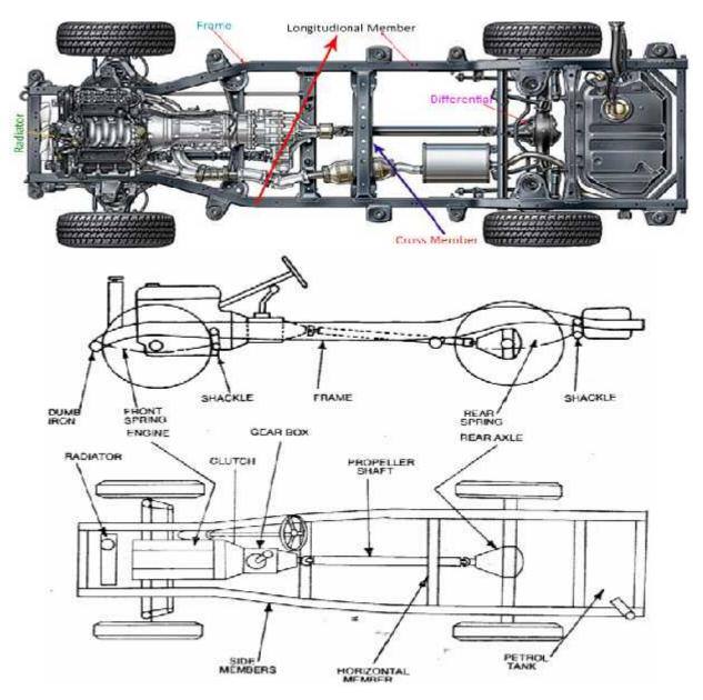
Differential- It is a device that splits the engine torque two ways, allowing each output to spin at a different speed. The differential is found on all modern cars and trucks, and also in many all-wheel drives Suspension System
