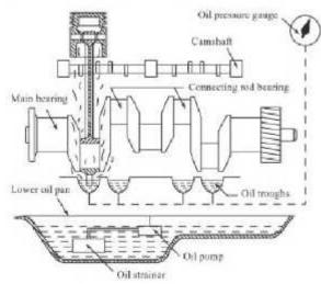
Splash and pressure lubrication system:
