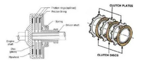
Main Parts of the Multi Plate Clutch
