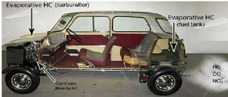
Emission sources in a gasoline fuelled car.
