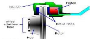
**1. Wheel Hub:** The disc rotor is attached to the wheel hub and it rotates with it. The wheel of the vehicle is bolted to the wheel hub.
