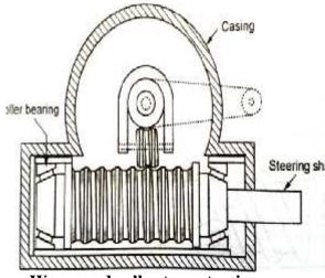
Worm and roller type steering gear
