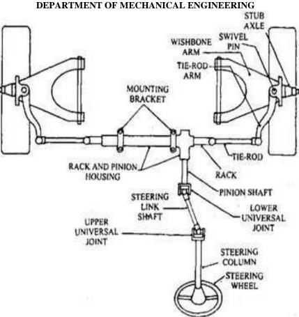
Rack-and-pinion steering linkage layout.
