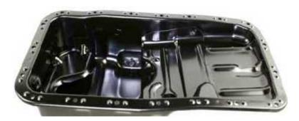
The oil pan serves as a reservoir for the storage, cooling and ventilation of engine lubricating oil. At the bottom of the oil sump, a drain plug is provided to drain out the dirty oil at the time of oil replacement. Generally, the sump is made of pressed steel sheet or aluminum alloy casting is used.
