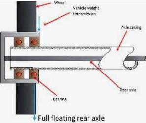
The axle shaft is connected to the drive wheel through a bolted flange. This allows the axle shaft to be removed for servicing without removing the wheel.
