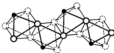
Fig. 22-C-10. A portion of an infinite chain of \text{MoCl}_5\text{O} octahedra that occurs in monoclinic \text{MoOCl}_3 . Solid and broken circles represent, respectively, upper and lower chlorine atoms; dots are oxygen atoms.
