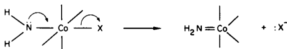
Fig. 28-4. How an amide group could promote the dissociation of another ligand X.
