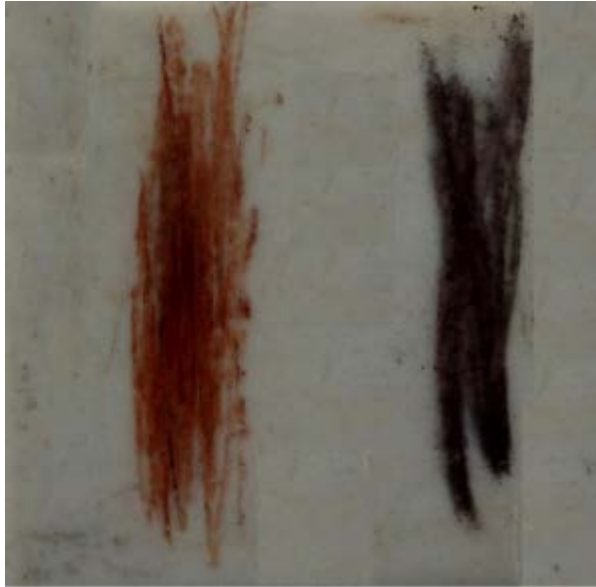
Figure 2.17 The streak colours of earthy hematite (left) and specular hematite (right). Although the specular hematite streak looks close to black, it does have red undertones that you can see if you look closely. [SE]
