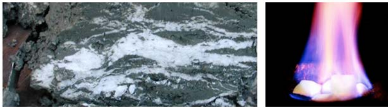
Figure 18.11 Left: Methane hydrate within muddy sea-floor sediment from an area offshore from Oregon. [ https://upload.wikimedia.org/wikipedia/commons/4/49/Gashydrat_im_Sediment.JPG ] Right: Methane hydrate on fire [ http://www.usgs.gov/blogs/features/files/2012/01/New-Image.jpg ]
