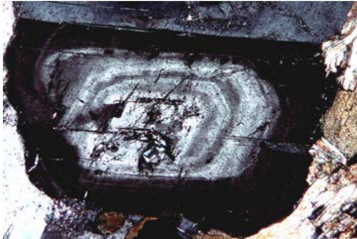
Figure 3.11 A zoned plagioclase crystal. The central part is calcium-rich and the outside part is sodium-rich: [Sandra Johnstone, used with permission]
