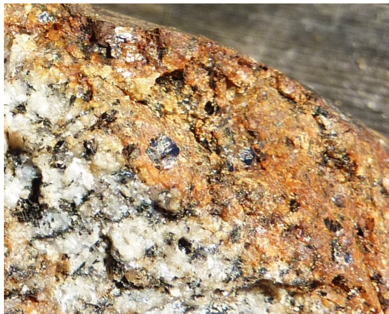
Figure 5.10 A granitic rock containing biotite and amphibole which have been altered near to the rock's surface to limonite, which is a mixture of iron oxide minerals. [SE]
