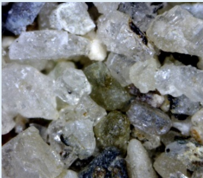
Angular quartz and rock fragments from a glacial stream deposit near Osoyoos, B.C. The grains are between 0.25 and 0.5 mm across.
