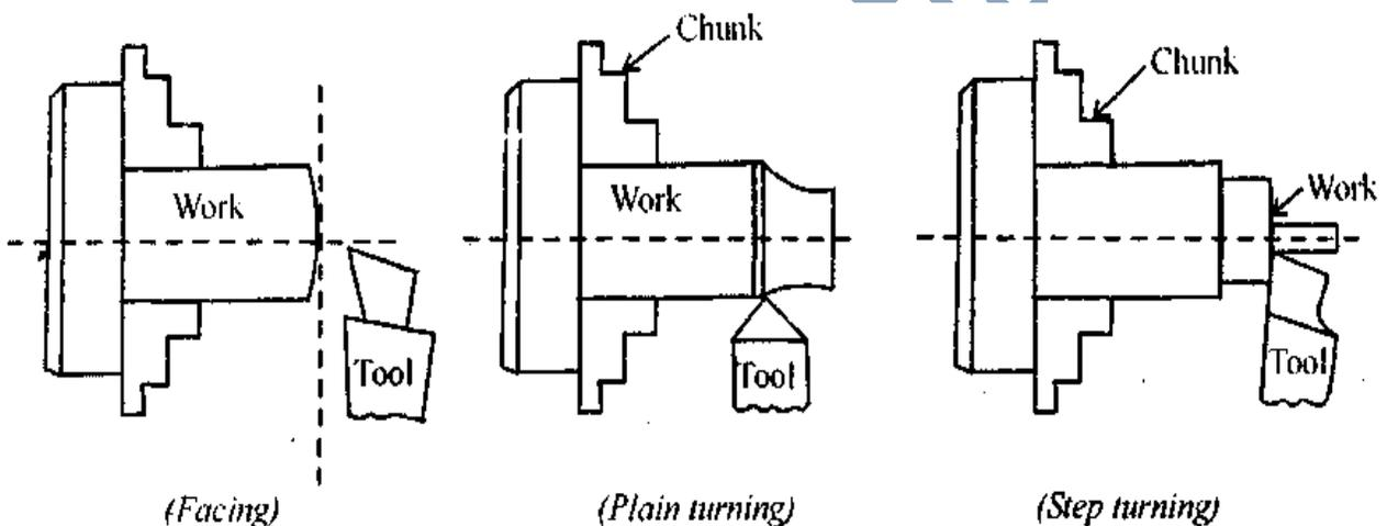
(iii) **Step Turning:** It is an operation of producing various steps of different diameters of in the work piece as shown in fig. This operation is carried out in the similar way as plain turning.
