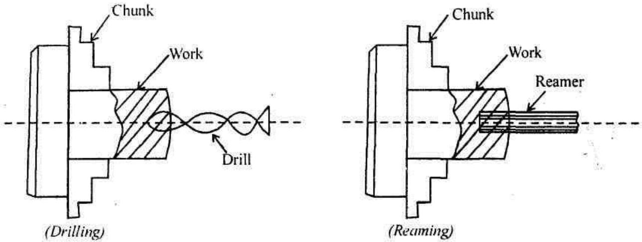
(v) **Reaming** : It is an operation of finishing the previously drilled hole. In the operation as shown in fig., a reamer is held in the tailstock and it is fed into the hole in the similar way as for drilling.
