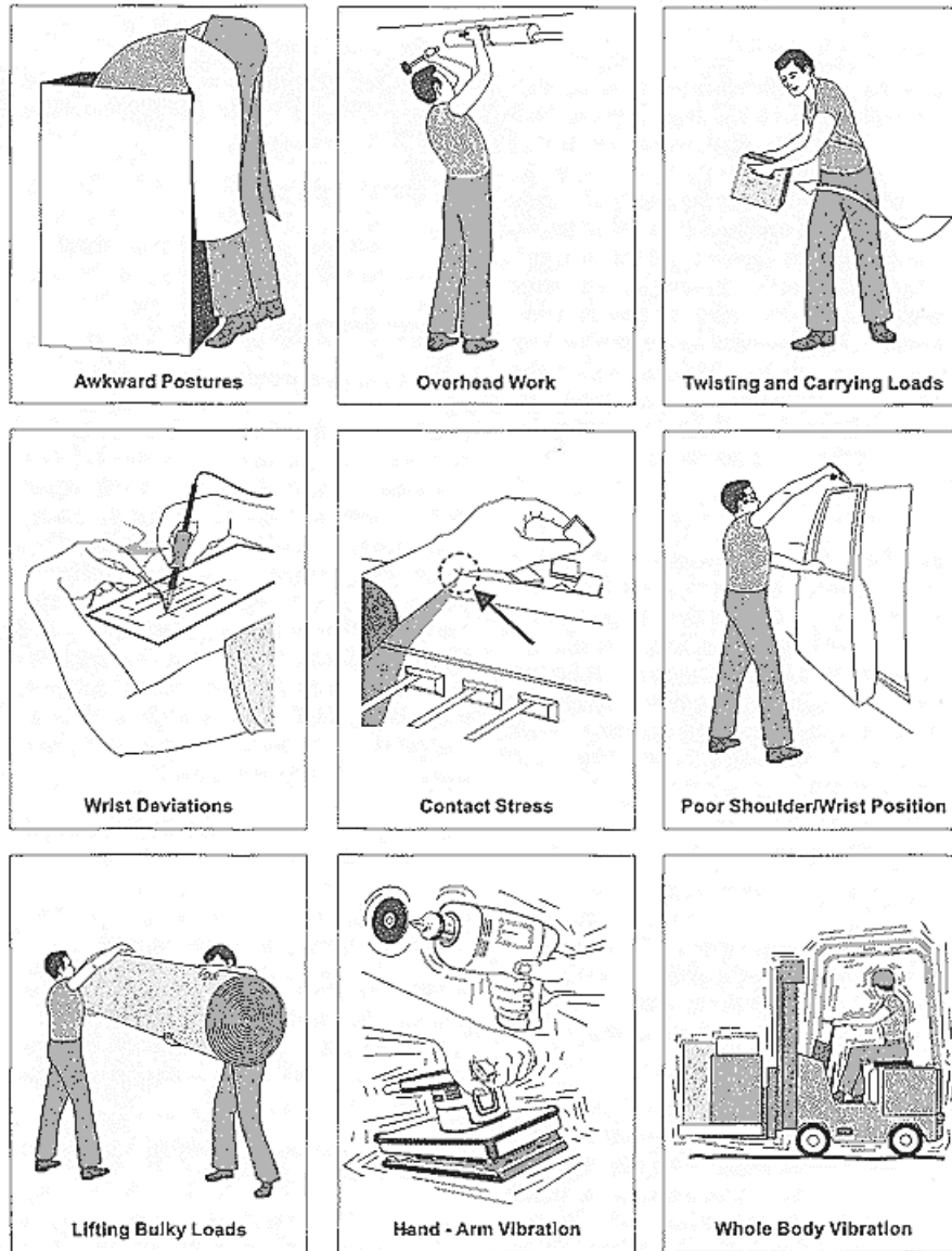
Figure 1. Selected risk factor conditions. (Illustrations adapted from UAW-GM Center for Health & Safety [1990]; Putz-Anderson V [1988]; Grant et al. [1995]; Canadian Center of Occupational Safety and Health [1988]; American Meat Institute and Ergo Tech, Inc. [1990].)
