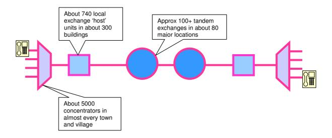
Figure 5: Telephone network architecture
