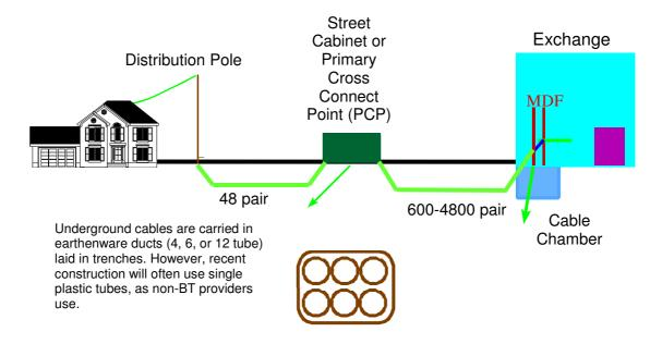
Figure 2: Typical layout of a local access network
